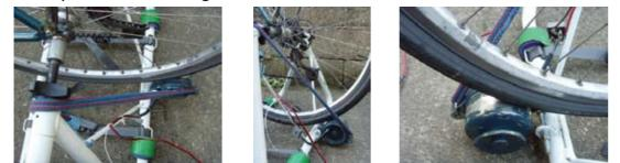
The dynamo is 24 Volt AC, which means we need some extra parts between it and the appliances we want to run (on either 12V DC or 240V AC). The first of these is a Bridge Rectifier (under  $\pounds$ 5). This converts the AC Voltage into DC. If you had a DC motor/dynamo you'd want a Diode here instead, to prevent current from travelling into the motor and making it spin ( $\sim f2$ ). The rectifier is the small grey box in the pictures above (most clear in the central picture).
