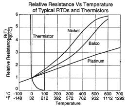
Platinum's resistance versus temperature function is accurately modeled by the Callendar-Van Dusen equation. This equation uses constants A, B and C, derived from resistance measurements at 0°C, 100°C and 260°C.
