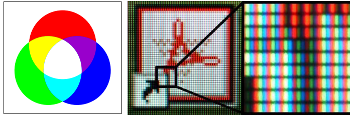
Figure 23: Red, green and blue are the primary additive colours in the RGB system. On the right is a close-up of a modern flat-panel computer screen. The image shows clearly how White is a result of mixing the three primaries. Each triplet or pixel is about 0.26 millimetres square.
