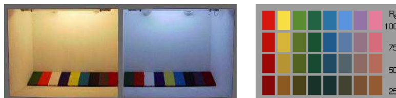
Figure 22: Left: A colour comparison box with test strips under different light; Right: Test swatches and their appearance under different CRI
