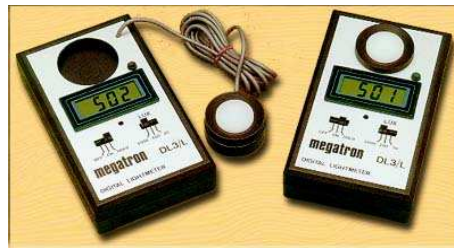
Figure 18: Illuminance meter (Image courtesy of Megatron [C1])
