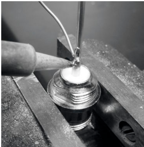
Figure 4.39: Solder the wire to the gold cup on the N connector.
