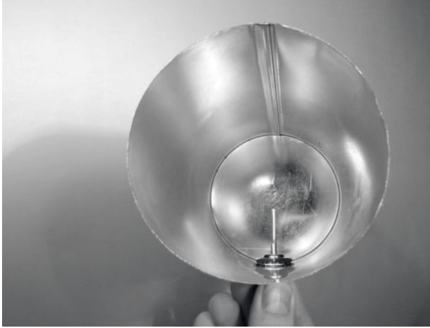
Figure 4.42: Your finished cantenna.
