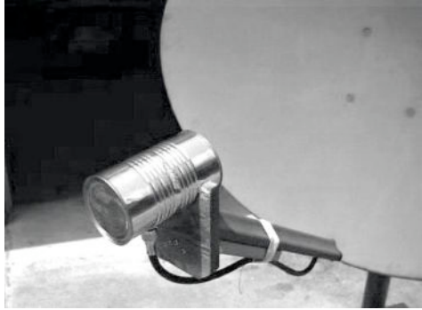
Figure 4.10: Feed horn made from a food can.
