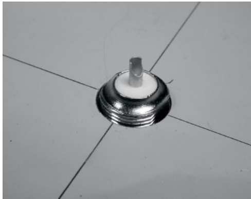
Figure 4.23: The N connector should fit snugly in the hole.
