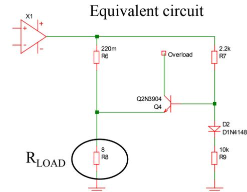
When a Class AB amplifier has a shorted load, the load current can ramp up rapidly. The voltage across the device is fixed to the bus voltage.
