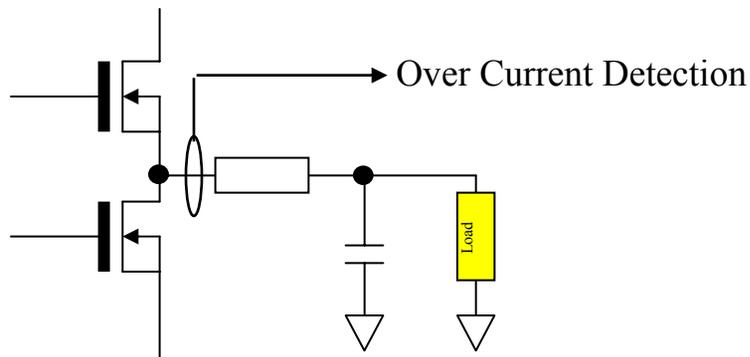
When a Class D amplifier has a shorted load, there still is a LPF inductor in between the load and the amplifier. Therefore, the load current ramps up at a rate of  $V_o/L$ .
