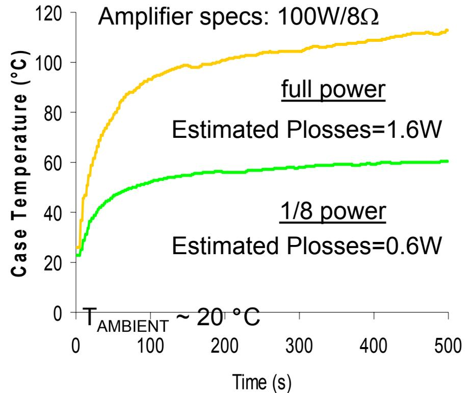
**Full Power: T<sub>c</sub>=104°C @ 5min ( $\Delta T_c=83^\circ\text{C}$ )**
