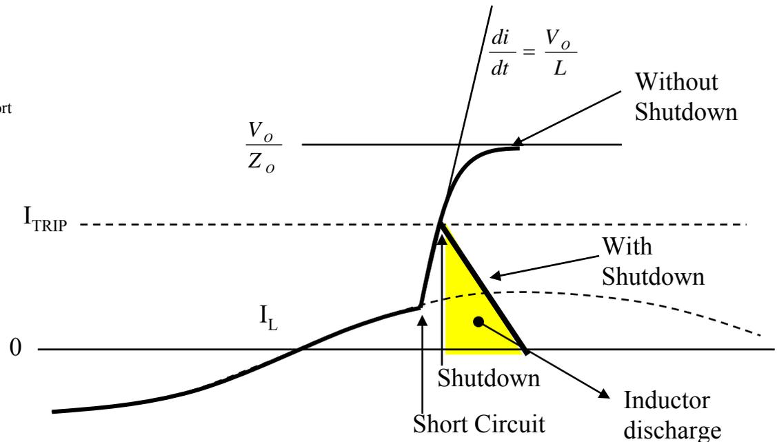
Now the Class D amplifier is driving an inductor in the LPF. Note that the audio frequency components induce quite large volt-second feeding into the inductor, causing excessive inductor current in the event of short circuit load.
