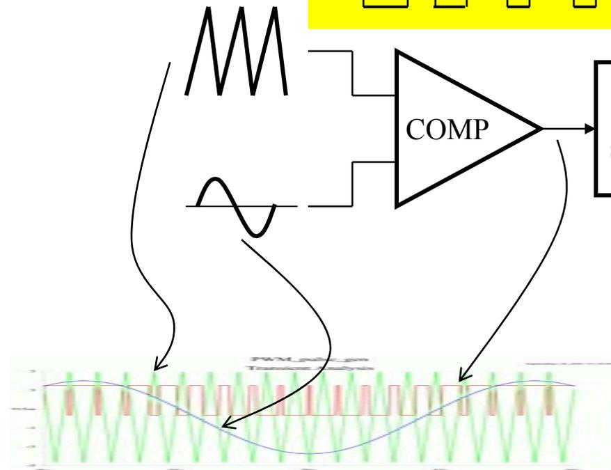
Using  $f_{PWM}=400kHz$  to modulate 25kHz sinusoidal waveform
