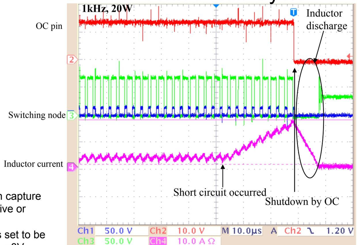
The bi-directional current sensing can capture over current conditions at either positive or negative current direction. In this demonstration, the threshold for  $V_s$  is set to be  $\pm 1V$  by setting  $OC_{SET1}=1V$  and  $OC_{SET2}=3V$ , which can be translated into 15A trip level with  $70m\Omega R_{DS(ON)}$ .
