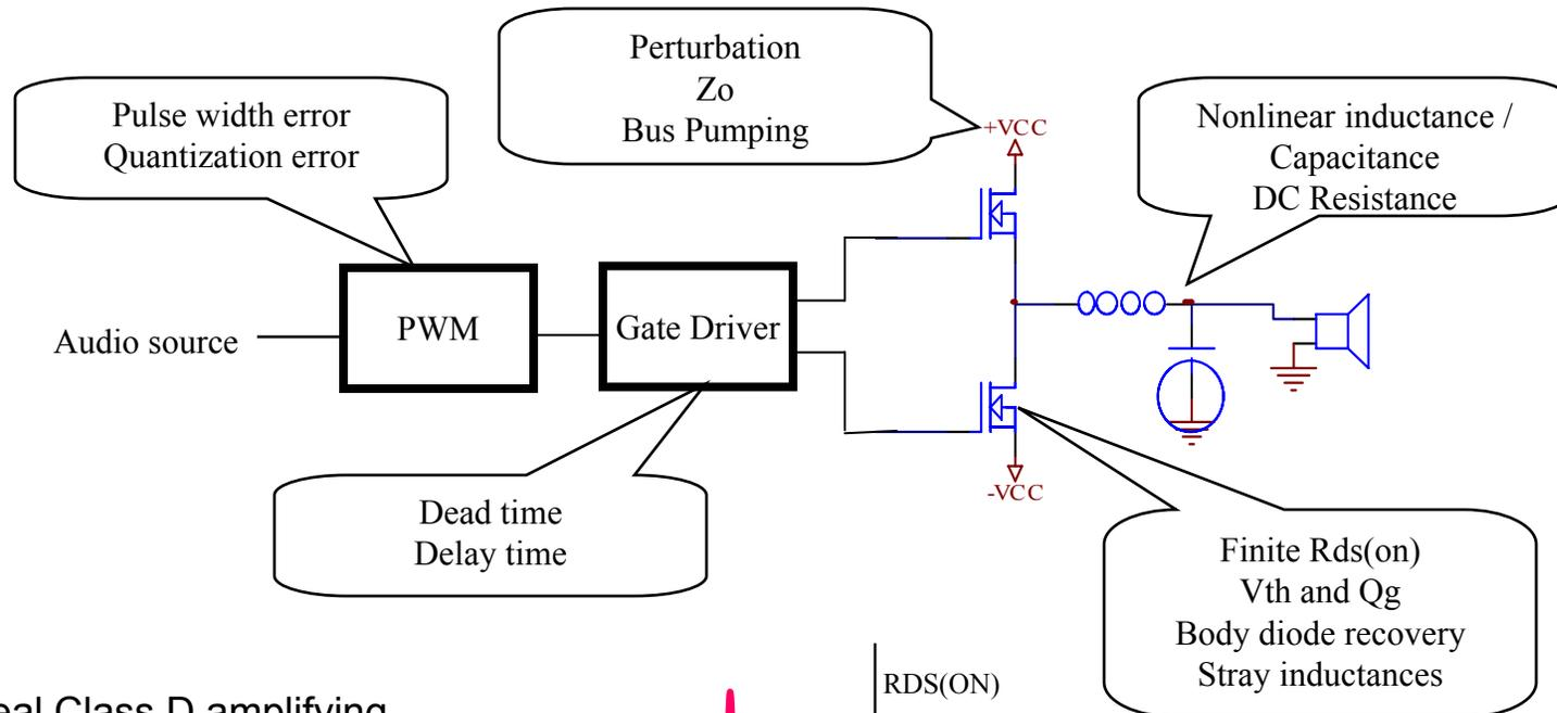
An ideal Class D amplifying stage has no distortion and no noise generation in the audible band, along with providing 100% efficiency. However, as shown, practical Class D amplifiers have imperfections that generate distortions and noise.
