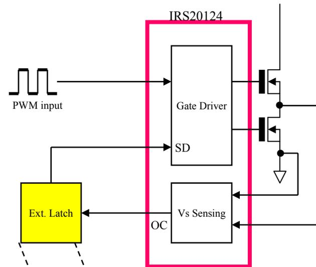
With the OC pin connected to DT/SD pin, the output signal out of OC at the event of over current will be removed by its output itself when the IRS20124 goes into shutdown mode. This could cause a hiccup in the protection sequence.
