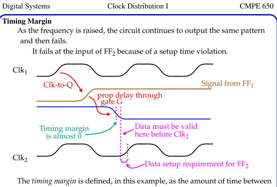
The *timing margin* is defined, in this example, as the amount of time between the emergence of signal from G and time when data for FF<sub>2</sub> must be valid. It is the slack remaining in each clk cycle.
