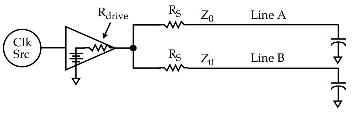
Here, the lengths of the lines *must be the same* and the *loads must be balanced*.
