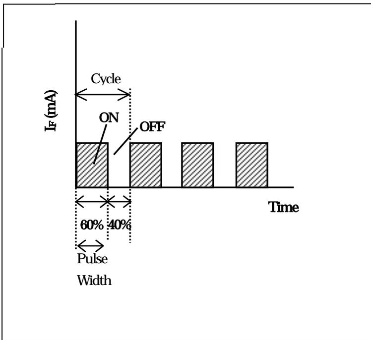
**Figure 5 : Pulse-width modulation (PWM)**
