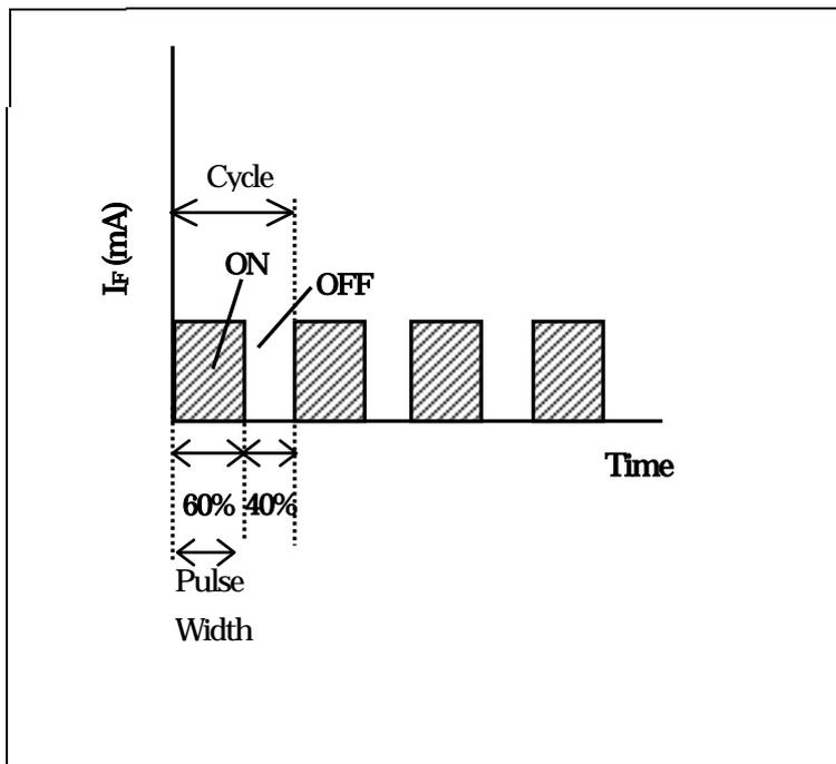
**Figure 5 : Pulse-width modulation (PWM)**
