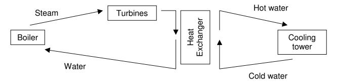
In chemical processes excess heat can be generated. This heat is removed using heat exchangers and cooling water which is cycled through a cooling tower.
