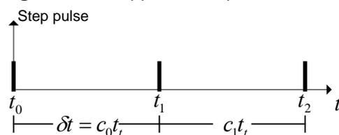
A counter generates these pulses, running at the frequency  $f_t$  [Hz].
