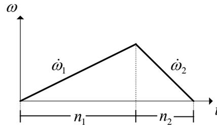
Moving a given number of steps, deceleration must start at the right step to end at zero speed. The following equation is used to find  $n_1$ :
