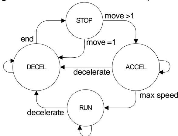
When the application starts or when the stepper motor is stopped the state-machine remains in the state STOP. When setup calculations are done, a new state is set and the timer interrupt is enabled. When moving more than one step the state-machine goes to ACCEL. If moving only 1 step, the state is changed to DECEL.
