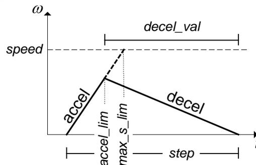
If  $max\_s\_lim > accel\_lim$  the acceleration is limited by deceleration start,  $decal\_val$  is then found by:
