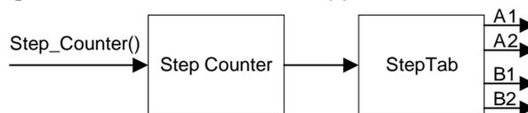
The step counter increments or decrements every time the function `Step_Counter()` is called. When using fullsteps, the counter value goes from 0 to 3, when using halfsteps, the value goes from 0 to 7. This value equals the different position in one electrical cycle in the stepper motor. The step counter value is used as an index for the step table, and correct signals is given to the stepper motor driver.
