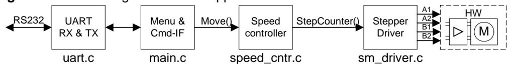
`main.c` has a menu and a command interface, giving the user control of the stepper motor by a terminal connected to the serial line.
