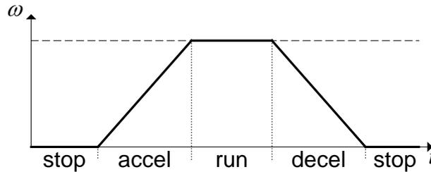
This behavior is realized with a state machine in the timer interrupt, shown in Figure 3-7.
