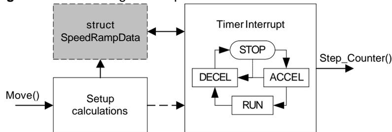
The function Move() first calculates all the parameters needed and stores them in the speed ramp data struct, then it enables the timer interrupt. The timer generates interrupts according to the desired speed ramp, and calls the function Step\_Counter() on each interrupt to move the stepper motor.
