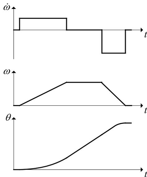
The time delay  $\delta t$  between the stepper motor pulses controls the speed. These time delays must be calculated in order to make the speed of the stepper motor follow the speed ramp as closely as possible.
