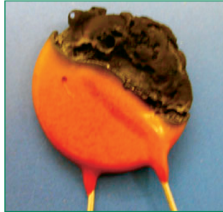
Figure 6a. Standard MOV
