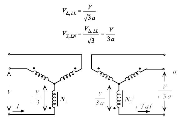
Comparing the voltages and currents of the primary and secondary windings, we see the that the equivalent turns ratio of the wye-wye configuration is
