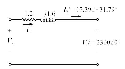
The resulting primary voltage  $V_1$  (line-to-neutral) is
