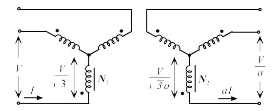
Note that the voltage across a wye-connected primary or secondary winding is the line-to-neutral voltage while the voltage across a deltaconnected primary or secondary winding is the line-to-line voltage. The magnitude of the complex three-phase power into or out of a three-phase transformer in a balanced system may be written as
