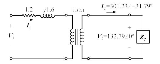
The secondary values can be reflected back to the primary according to the modified turns ratio a'.
