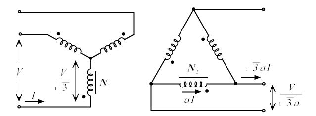
The line-to-neutral voltages across the windings of the equivalent wyeconnected secondary are found by dividing the line-to-line voltages across the windings of the of the delta-connected secondary by  $\sqrt{3}$ .
