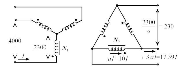
The given equivalent impedance for each transformer is referred to the LV winding (secondary). This impedance referred to the HV input winding is
