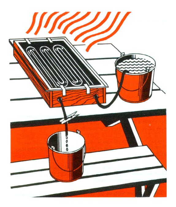
Notice that after a while, the water trickling from the tubing will be warmer than the water siphoning into the collector. Why? You're right. Solar energy absorbed by the tubing is transferred to the water, thereby heating the water.
