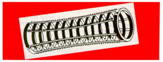
Making a fuel cell would be easy if we had the right materials. Trouble is, the right materials are either dangerous or difficult to get in small quantities. So let's take an easier path. Let's build a device that is considered to be a form of fuel cell. It uses zinc as the fuel (one electrode), air as the oxidant (the other electrode), and salt water as the electrolyte.
