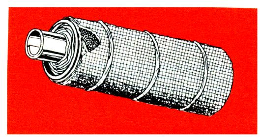
On a portion of one of these strips, spread all the graphite paste (messy, isn't it?). You need cover only the first 3" of length, but cover the entire width of this 3" portion. Then place the mesh tube on the graphite and wrap the strip around the tube. The graphite will be facing the meshwork, of course.
