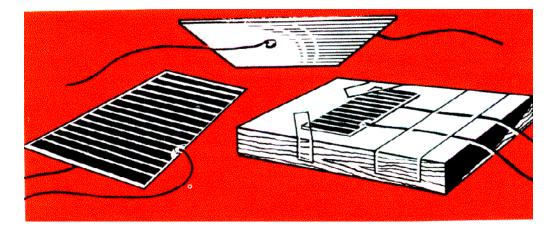
Finally, tape the cell and wires to your block of wood so that you can handle it conveniently.
