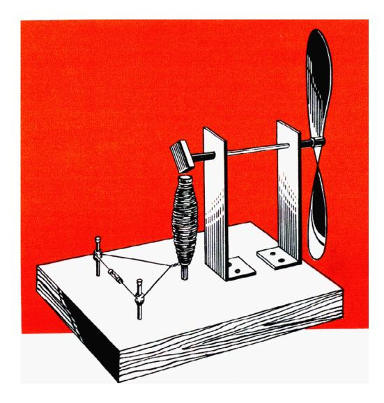
The shaft is supported by the two tin-can strips. Fold them in half lengthwise for added stiffness. Then bend about  $\frac{3}{4}$ " for the base. Nail them to the wood block, in line with the upright nail.
