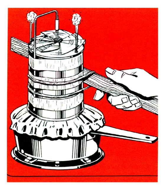
12. Bring the water to a boil. When steam starts jetting from the hole, lower the can over the hole, using the stick as a handle. The steam pouring from the two holes in the soup can will start the turbine spinning merrily.
