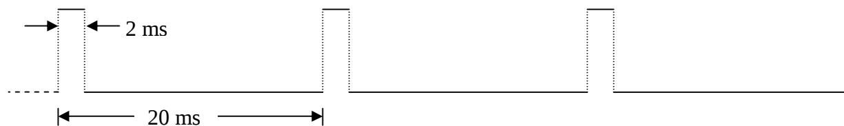
Figure 1: Pulse waveform with 10% duty cycle
