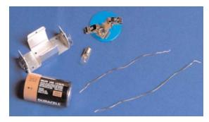
Step one: Insert the light bulb in the bulb socket.
