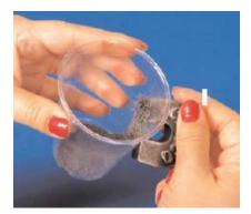
the magnetic force has to travel so far, the magnetic field on the surface is fairly weak. For the field to be able to affect your compass, it's important to have a lightweight magnet (needle) and frictionless bearing (cork).
