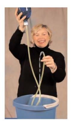
Let's think about what is happening as we change the height of the tubing in relation to the level of the water in our bottle. As we raise the tubing higher we decrease the potential for the water (or electrons) to flow through the tubing. As we lower the tubing we increase the potential for flow. This change in potential relates to another electrical term called voltage.
