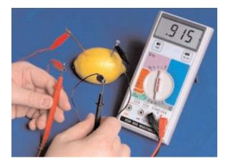
**Step four:** Attach alligator clips to each electrode and then connect the alligator clips to the multi-meter.
