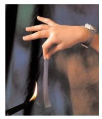
molecules generated by the heat get near the tape, opposite charges are attracted to the tape
