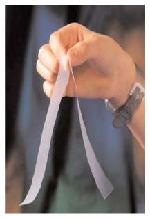
**Step One:** Take two strips of tape and place the non-adhesive sides together to show how they repel each other.
