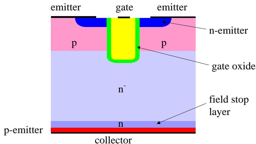
Figure 1.15 IGBT-cell with trench-gate and field stop layer
