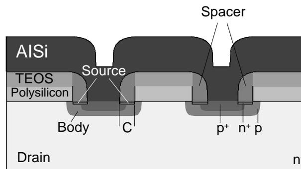
Figure 1.14 Double-implantation gate structure (Siemens S-FET) [298]
