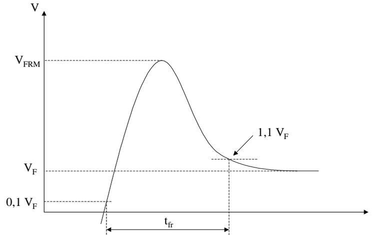
Figure 1.18 Turn-on behaviour of power diodes
