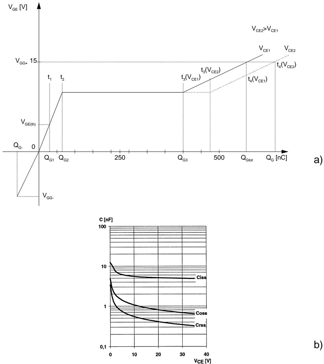
Figure 1.13 a) Extended IGBT gate charge characteristic for gate control between  $V_{GG+}$  and  $V_{GG-}$ .
