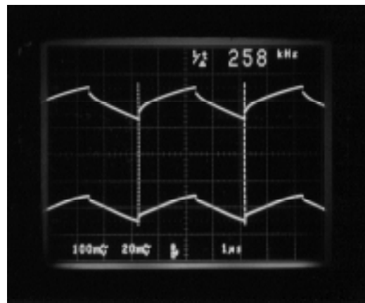
Figure 8: Bottom- A 260kHz disturbance appears on the input line(100mV/div) Top-This disturbance is transmitted to the output of LM2596(20mV/div)
