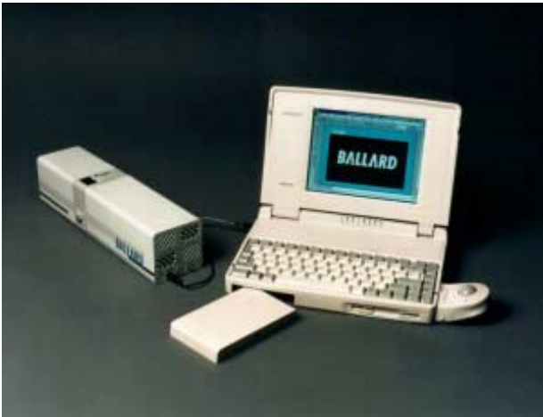
Figure 5. Portable fuel cell for use with laptop computer (photo courtesy of Ballard)
