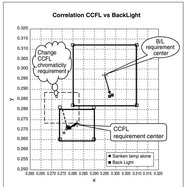
\* In the above figure, we can aim at the center value of B/L chromaticity requirement by shifting the center value of the CCFL requirement in a manner that the deviation of CCFL chromaticity from the center of the standard equals the deviation of B/C chromaticity from the center value of the requirement.
