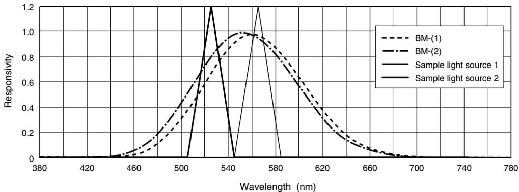
Instrumental error between two BMs can increase, even when measuring a light source with the same peak wavelength. For example, in the figure below, instrumental error is greater when sample light source 4 was measured rather than when sample light
