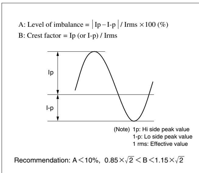
When the lighting waveform is asymmetrical, the  $Hg^+$  ions in the discharge space are strongly attracted to either of the two electrodes, resulting in uneven mercury migration.
