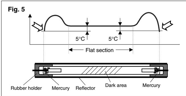
**4-3 Failure Mode due to Irregular Lighting Waveform**
