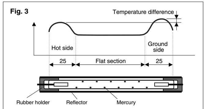
(1) In the case that temperature gradient exists on the flat section between electrodes (Fig. 4)
