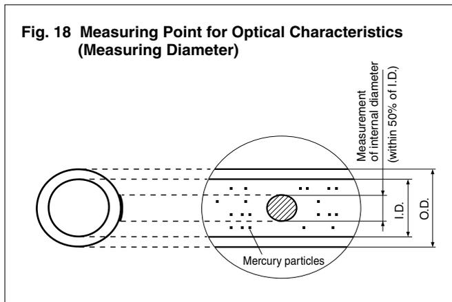
**Fig. 18 Measuring Point for Optical Characteristics (Measuring Diameter)**
