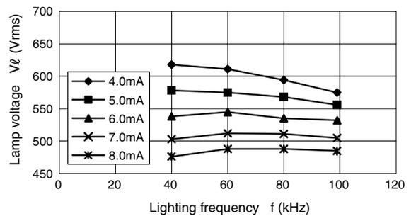
**Fig. 12 Lighting start voltage - lighting frequency characteristics**
