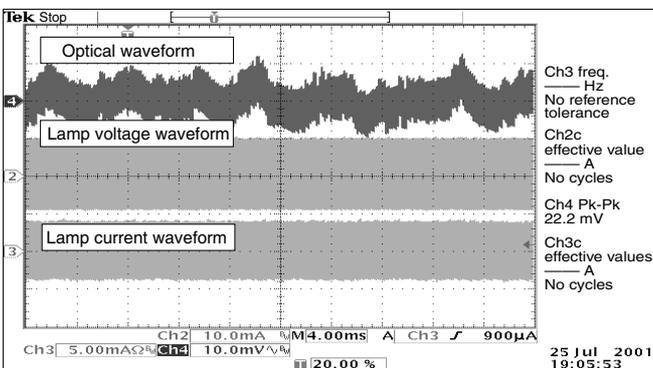
The dimming range changes because the lamp surface temperature varies with heat dissipation of the system and the lighting waveform of the inverter. Before setting the dimming range, check the optical waveform that appears under the operating conditions of the lowest lamp surface temperature (low temperature, minimum dimming) using the actual system.
