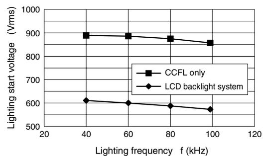
[Cautions] Lamp voltage and Lighting start voltage of a CCFL used as an independent lamp are different from those of a CCFL used in a system.
