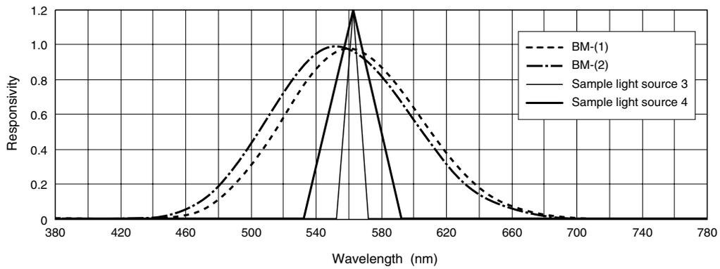
As described above, the instrumental error is closely related to the spectral characteristics of the instrument and the light source to be measured. This also applies to the tristimulus values XYZ.
