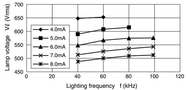
**Fig. 11 Lamp voltage - lighting frequency characteristics**
