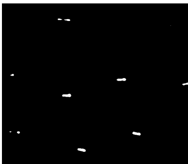
Fig. 17d. Domains in 0.13 mm (YbTbBi)IG film with about 100 mT applied perpendicularly to the film.
