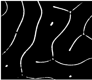
Fig. 17c. Domains in 0.13 mm (YbTbBi)IG film with slightly less than 100 mT applied perpendicularly to the film. Some of the domains from a and b are still visible.
