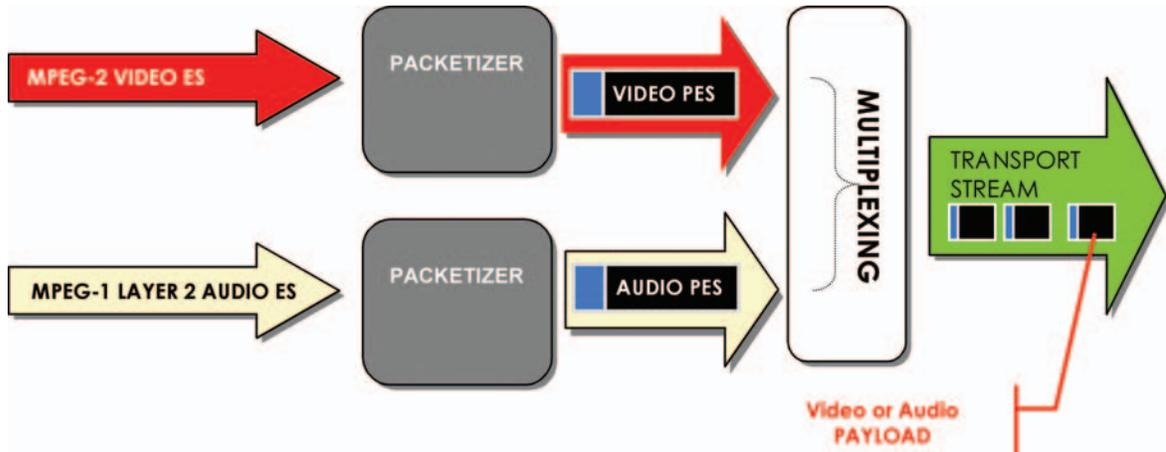
Thus, the video-PES and audio-PES streams are multiplexed to form a single Transport Stream. The transport stream packets have a fixed 188 Byte packet size. The PES packet size is variable e.g. 2048 Byte; much longer than a transport packet. Thus, each PES packet is subdivided into multiple TS packets as described below.
