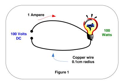
To work out a close approximation of how fast an electric current is flowing in any conductor we need to know the *charge carrier density* on the material carrying the current. In other words the number of free electrons per cubic measure.
