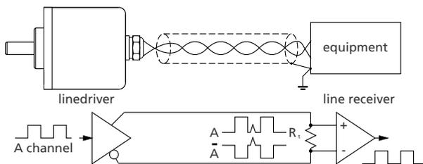
The value of the terminating resistance should ideally equal the characteristic impedance of the line. A good value is 120  $\Omega$  for a twisted-pair or parallel-wire connection.
