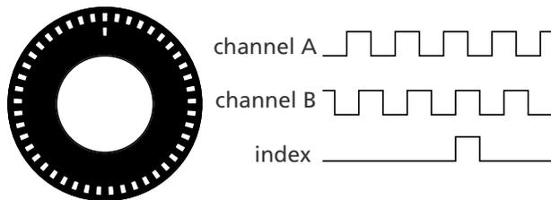
As a rule, a second track is added to generate a signal that occurs once per revolution (index signal), which can be used to indicate an absolute position.
