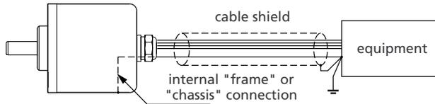
For cable lengths of more than 6m (20 feet), linedrivers are recommended. These are devices that meet the requirements of EIA standard RS-422-A, Federal Standard 1020 and DIN 66259 (Teil 3). Linedrivers have complementary outputs (= signal output and the inverse signal output) and high current capability for driving balanced lines such as twisted-pair or parallel-wire transmission lines.
