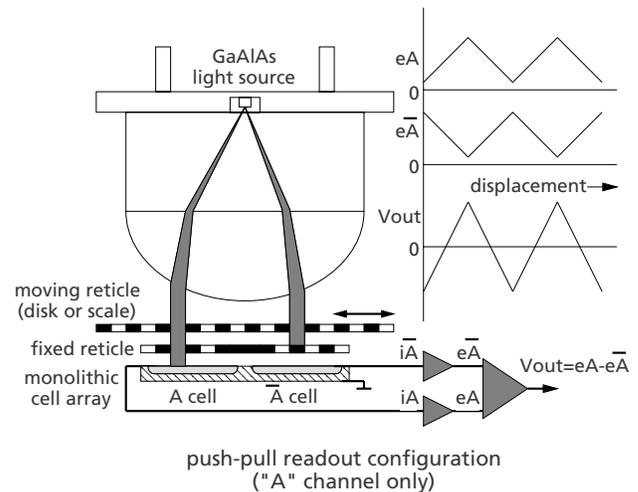
All optical encoders are inherently analog devices. The disk or scale moves with a finite speed and gradually cuts off or admits light to the photo-elements.
