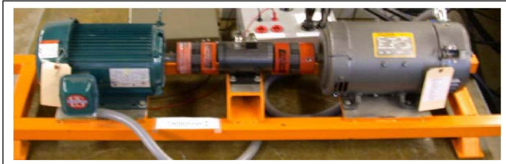
Fig. 6.1: 5 Hp DC Machine coupled to an Induction Machine
