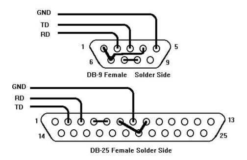
This solder side view shows how to wire the DB-9 (female) or DB-25 (female) connector for an IBM PC compatible computer
