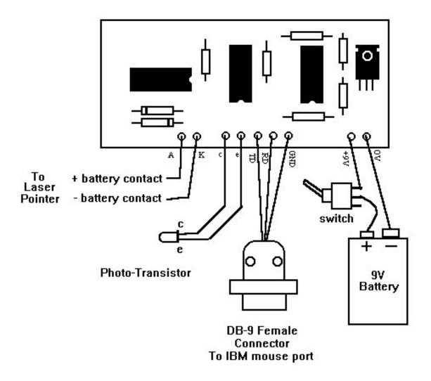
Connections to the external components are shown here for both the transceiver and the transmitter.
