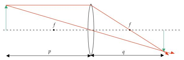
The analysis (in the paraxial ray approximation) gives the same formulas for location of the image (and for lateral magnification) as we had for mirrors.
