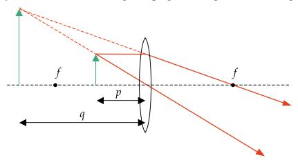
The image is erect and enlarged. An example of this is production of an enlarged virtual image by a magnifying glass.
