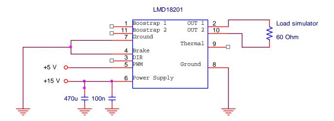
**STEP 15.-** Connect Pin 3 (DIR) to +5 V. Using a Multimeter, estimate the current through the load by measuring the voltage drop. We need to use the multimeter instead of the oscilloscope because none of the load terminals are grounded.
