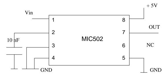
Pin 1 is the input voltage to the system, where the output of the Hall Effect sensor is connected. However, to characterize this chip, we will use an adjustable DC source connected to this Pin.
