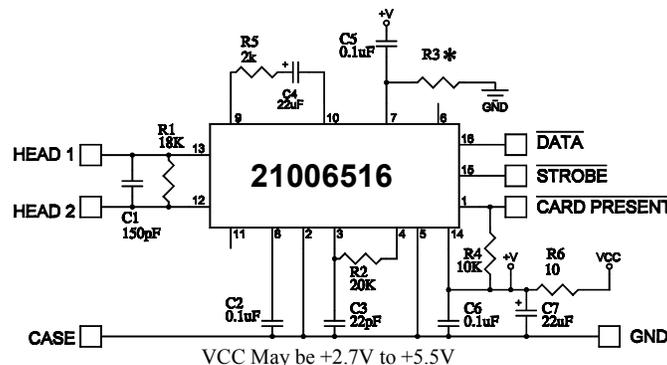
Tolerances: Resistors ±5%; C1, C3 ±5% NPO; other capacitors non-critical.
