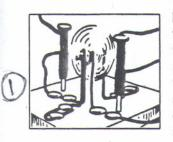
The finished motor shown to the left can be built with the following commonplace tools and materials: eight thumbtacks, three 2-inch paperclips, two 3 1/2 inch nails, needle-nosed pliers, electrical or adhesive tape, a wooden board about five inches square, about 20 feet of No. 20 insulated copper wire and a knife or sandpaper to scrape the ends with. Two 1 1/2 volt dry cells provide an adequate power supply.
