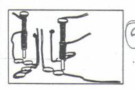
Step 10. Fit the axle of the rotor into the loops of each support so that the rotor's commutators, when twirling, will make contact with the brushes. Twist the end of the 6-inch tail from the second nail around the 9-inchwire from the first nail. The 9-inch wire from the second nail will connect with the dry-cell terminal. Link the free end of the 12-inch wire to the opposite dry-cell terminal and the circuit is complete.
