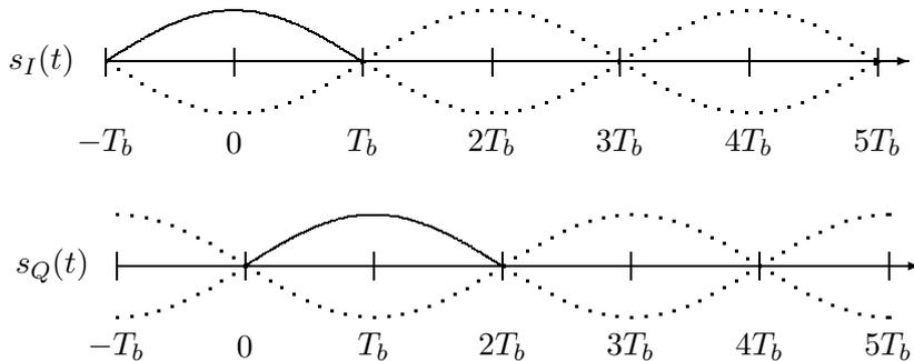
Figure 5: IN-PHASE AND QUADRATURE COMPONENTS.
