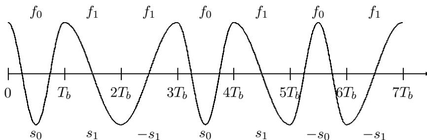
Figure 3: EXAMPLE OF AN MSK SIGNAL.
