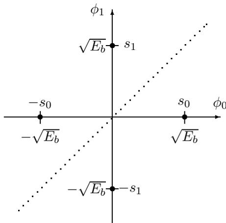
Figure 4: SIGNAL SPACE DIAGRAM WHEN DECODING MSK AS BFSK.
