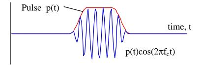
Now p(t) is made up of an infinite number of frequencies between 0 and W; consider what happens to **any one** of these frequencies say  $cos(2\pi f_0 t)$  when it is multiplied by the carrier frequency.
