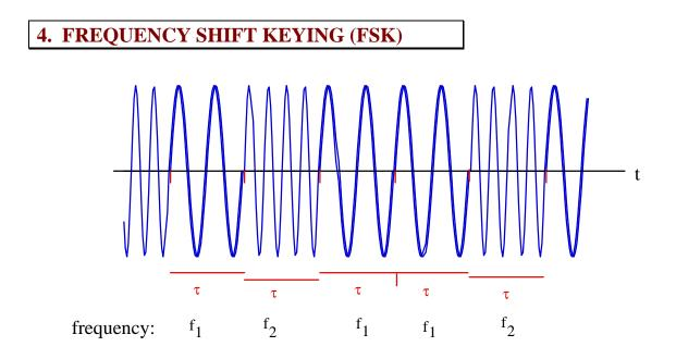
In this type of modulation scheme for *two-level pulses* we *always* put out a pulse p(t) that is amplitude modulating a carrier frequency, whether the data digit is a 1 or a 0, but we distinguish between the two digits by using **two** slightly different carrier frequencies  $f_1$  and  $f_2$ .
