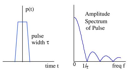
For train of such pulses with individual amplitudes corresponding to some *arbitrary* data stream, to receive each pulse individually at the receiver, bandwidth required is also W. With this bandwidth we can transmit W pulses/second (each pulse of width τ=1/W).
