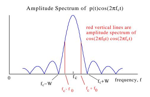
• Amplitude modulation of the carrier by the pulse results in an amplitude spectrum approximately contained between frequencies  $f_c$ -W to  $f_c$ +W. The total bandwidth is now 2W, centered at  $f_c$ .
