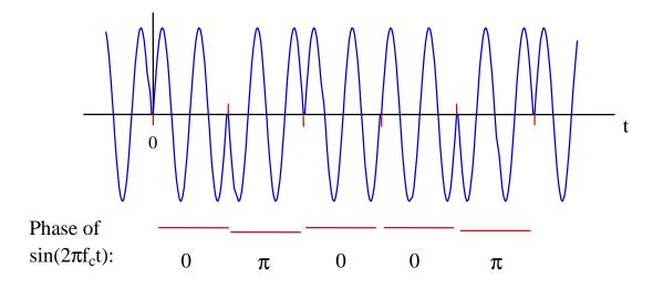
[We can equivalently think of the above as showing a pulse train with a carrier  $\cos(2\pi f_c t)$  in which the carrier phase is either  $-\pi/2$  or  $+\pi/2$ ; note that  $\cos(2\pi f_c t - \pi/2) = \sin(2\pi f_c t)$  and  $\cos(2\pi f_c t + \pi/2) = -\sin(2\pi f_c t) = \sin(2\pi f_c t + \pi)$ . In both cases the phase difference between the two alternatives is  $\pi$ .]
