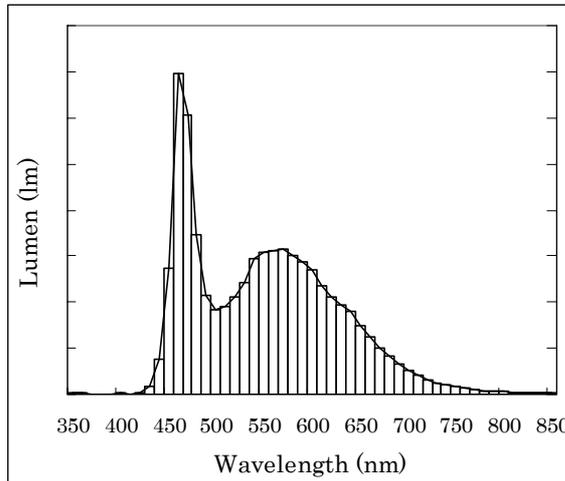
Figure 4: Spectral Distribution of White LED Light
