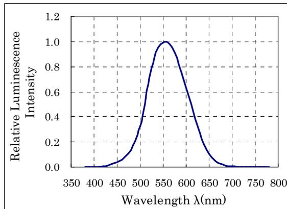
Figure 3: Standard Luminous Efficiency
