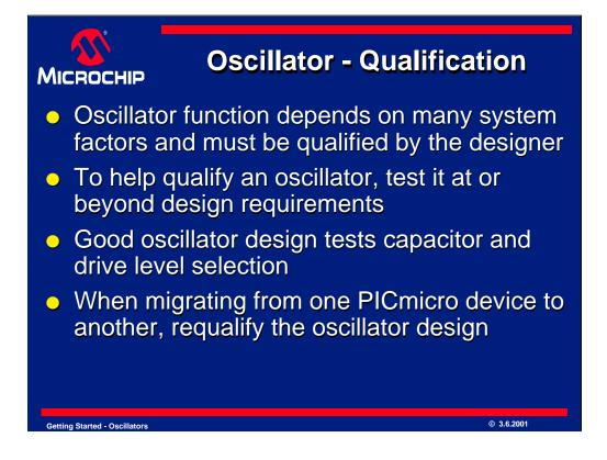
When an oscillator is designed, it should be qualified. The purpose of qualifying and requalifying an oscillator is to ensure it will work under all the conditions where it is expected and specified to perform. Oscillator designs should be tested just like your software and other hardware.
