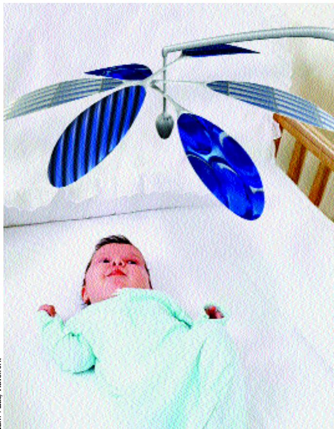
Figure 3. This award-winning baby mobile uses lightweight organic light-emitting diodes to realize images and sounds in response to gestures and speech of the infant.
