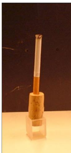
**Figure 6.** A glowing cigarette is attached to a piece of cork using a toothpick. If this is unstable, the cork may be squeezed into a holder.
