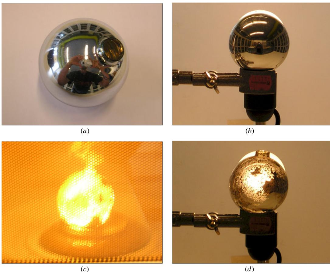
**Figure 3.** (a) Coated open glass sphere, usually used as a decoration on Christmas trees. Parts (b) to (d) correspond to the situation before (b), during (c) and after (d) treatment in the microwave. In the set-up of (b) and (d) the sphere is placed in front of an operating light bulb in order to demonstrate that in (d) a large part of the coating has evaporated, since the sphere has become transparent.
