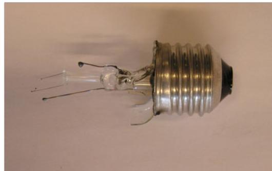
**Figure 10.** The filament and large parts of the support wires have evaporated.
