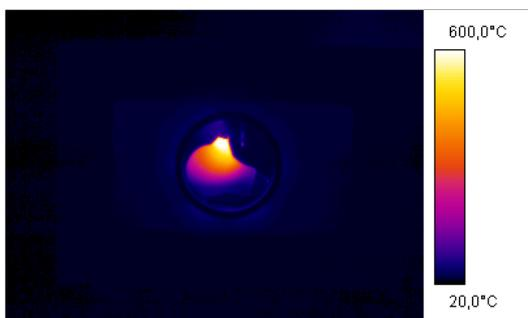
**Figure 12.** Infrared image directly after the explosion with surface temperatures at the top being above 620 °C.
