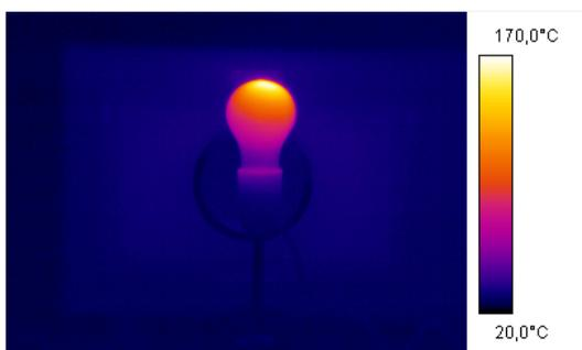
**Figure 11.** A 100 W light bulb after two minutes of operation.
