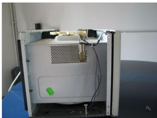
**Figure 7.** A microwave oven is illuminated by a light bulb behind a metal grid, e.g. at the side of the cavity (in this case, the microwaves are coupled in from the top).
