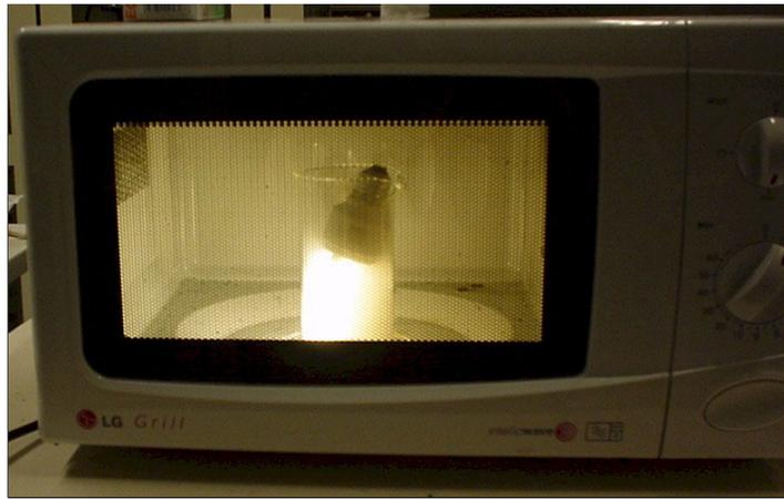
**Figure 13.** A discharge lamp (energy-saving lamp) during operation of the microwave.
