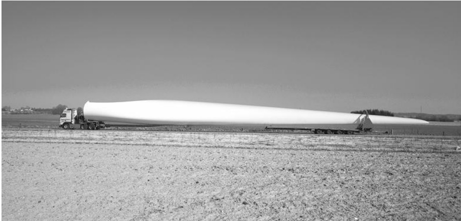
Figure 2.3: LM Glasfiber 61.5 meters blade developed for 5 MW turbines. Reproduced from [46].
