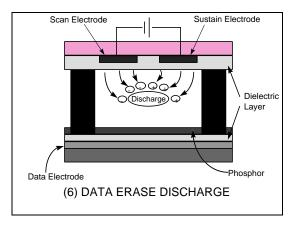
By repeating steps 2 through 6 the color PDP can create an image according to the input signals which are led to the driver circuits and these driver circuits instruct the sustain, scan and data electrodes.
