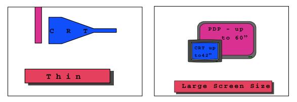
Why is Plasma suited to large screen sizes? It is relatively simple to manufacture in comparison to an LCD panel due to its less complex structure and wider spacing tolerances between front and rear substrate layers.
