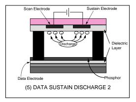
6. When lower voltage than the sustain high voltage is applied between the sustain electrode and the data electrode small discharges are created in the selected cells. These small discharges absorb the wall charge into the cell and the wall charge is erased.
