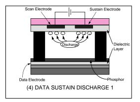
5. Continue to apply reverse polarity sustain high voltage between Sustain electrode and Scan electrode for selected cells to continue discharge and emit visible light.
