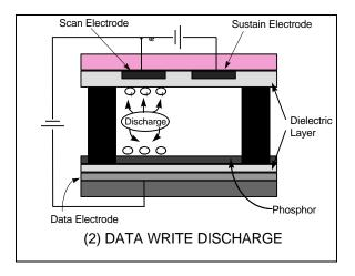
3. After the discharge is finished, charges remain on the surface of the dielectric layer in the selected (discharged) cells. These charges are called the "wall charge".
