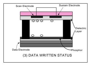
4. Apply sustaining high voltage between Sustain electrode and Scan electrode. The electric field created by this sustain high voltage does not exceed the threshold required to create a gas discharge but the additional electric field made by the wall charge causes gas to discharge. By this method only selected cells are lit by applying the sustain high voltage. After the discharge is finished reverse polarity wall charge remain only on the dielectric layer of the selected cells.
