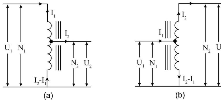
**Figure 15.7:** Autotransformers: (a) step-down; (b) step-up.
