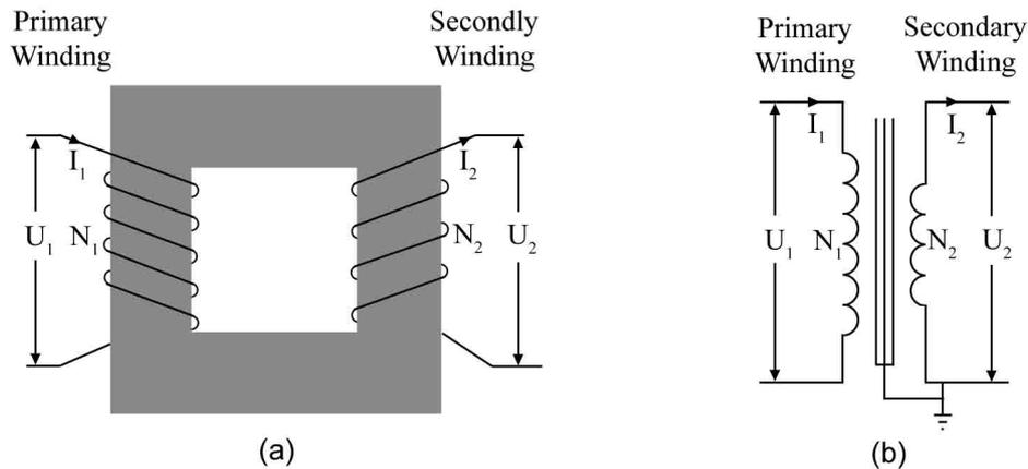
**Figure 15.1:** (a) a simple transformer; (b) the circuit diagram for a simple transformer.
