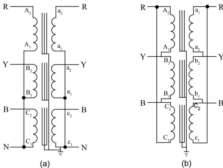
**Figure 15.3:** Three-phase transformers similarly connected: (a) star-star - for the primary and secondary one end from each winding is connected together forming a neutral; (b) delta-delta – one end of each winding connected to the next winding.
