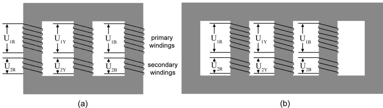
**Figure 15.6:** three-phase transformer construction: (a) core-type, three limb transformer and; (b) a shell-type five limb
