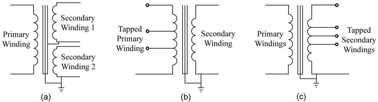
**Figure 15.2:** Methods for obtaining multiple voltages from a single transformer: (a) multiple secondary windings; (d) tapped primary winding; (c) tapped secondary winding.
