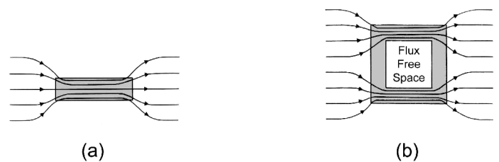
Figure 5.5: (a) a ferromagnetic material in a magnetic field; (b) a ferromagnetic material being used as a magnetic shield.
