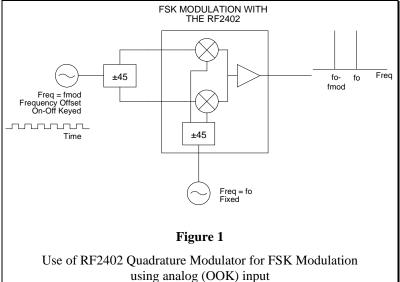
The LO is applied as a fixed-frequency oscillator at one of the desired output frequencies  $f_o$ (corresponding to data input "0"). Note that for this case, the I/Q signal inputs need a DC offset relative to the I/Q reference ports to achieve carrier feedthrough.
