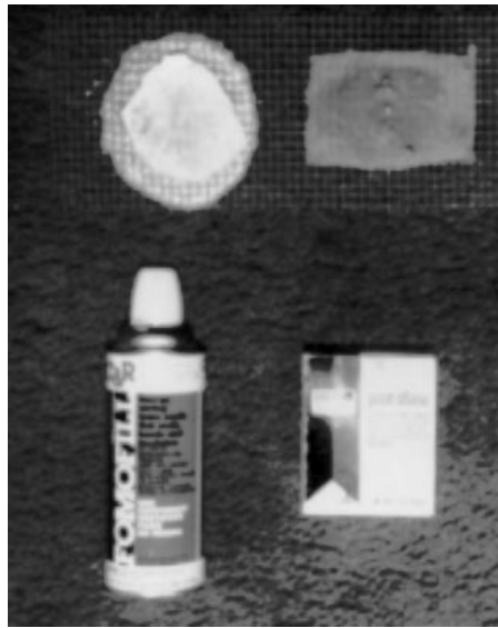
Fig. 10. Frequently used patching materials on 1/4-inch woven hardware cloth backing. Fomofill®, Pour Stone®, Fix-all®, and Custom Plug® are shown as examples of the many materials available.
