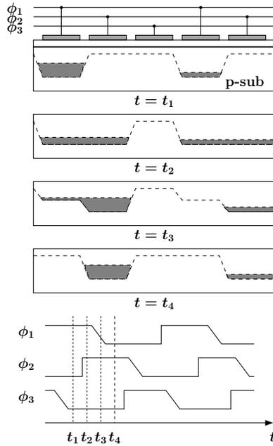
Potential wells and timing diagram during charge transfer
