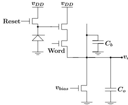
in steady state assuming charge  $Q$  accumulated on the photodiode at the end of integration and ignoring the voltage drop across the access transistor, the output voltage
