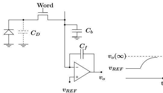
in steady state, assuming charge  $Q$  accumulated on the photodiode at the end of integration (and ignoring “feedthrough” voltage added when the reset transistor is turned off and opamp offset voltage), the output voltage
