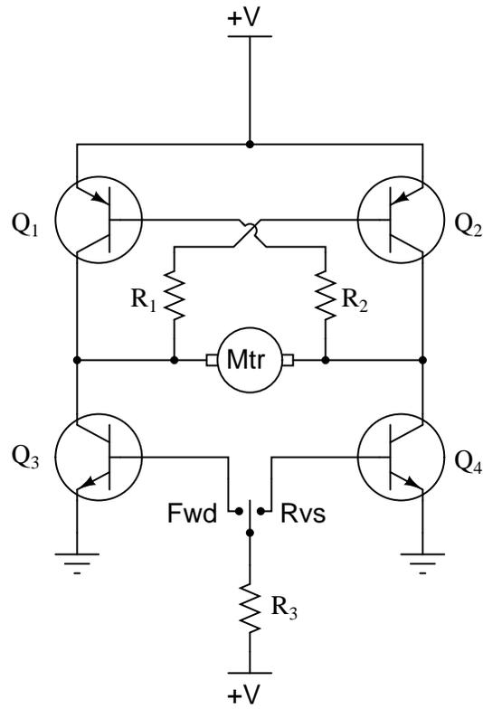
At any given moment, how many transistors are turned on and how many are turned off? Also, explain what would happen to the function of the circuit if resistor R1 failed open.
