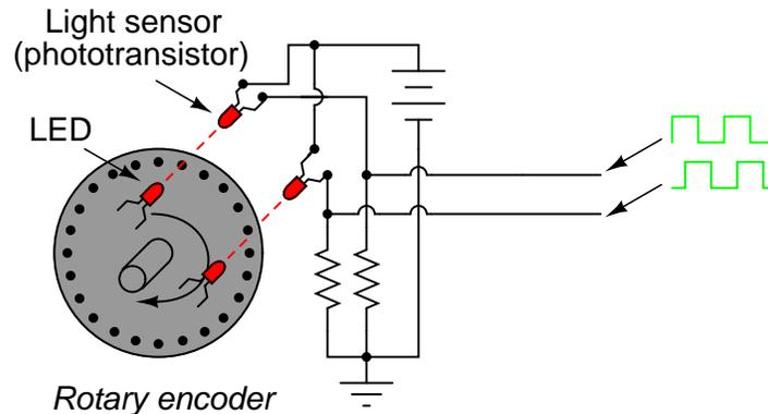
The two LED/phototransistor pairs are arranged in such a way that their pulse outputs are always 90° out of phase with each other. Quadrature output encoders are useful because they allow us to determine direction of motion as well as incremental position.
