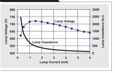
operating principle of the CCFL backlight power-supply controller. At turn-on, the lamp is an open circuit, so the PZT operates on the high-gain, high-impedance load line shown in Figure 7. Since the exact strike voltage and operating frequency are not known, the controller applies
