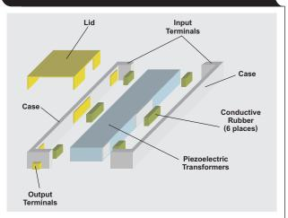
The mechanical resonant frequency,  $\omega_0$ , of the PZT is also dependent upon geometry and material.
