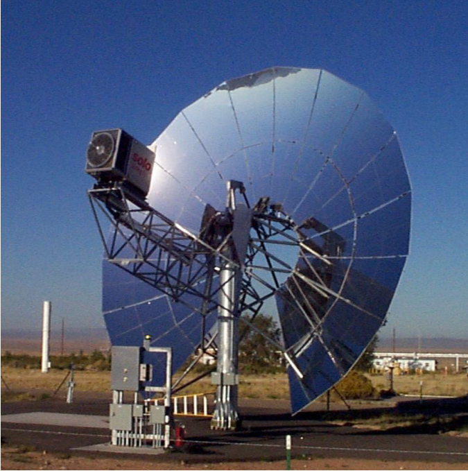
This Stirling engine is driven by a parabolic dish that collects and concentrates the sun into a heat source to run the engine and produce power.
