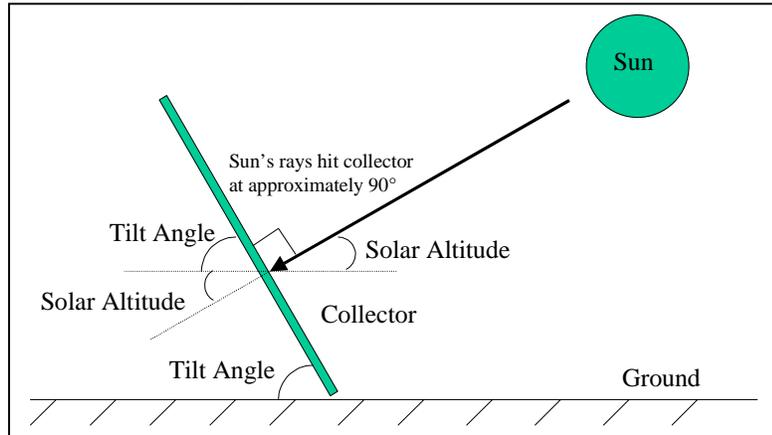
**Figure 4 Solar Collector Tilt Angle**
