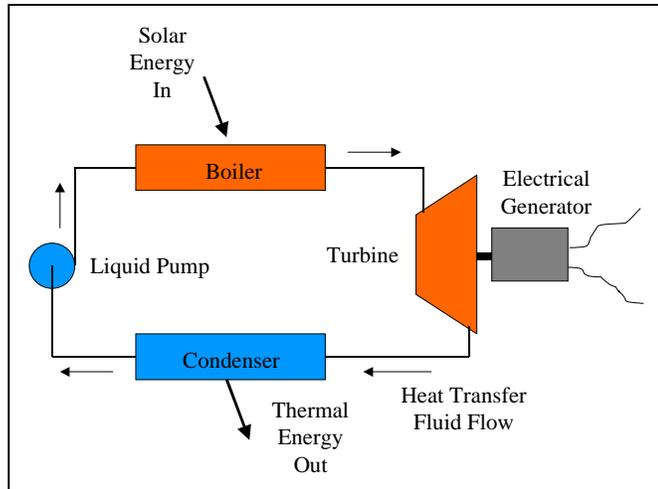
**Figure 11 Thermal Electrical Generation Cycle**
