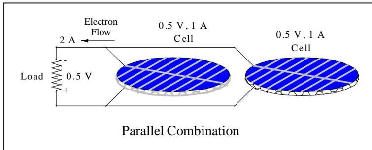
**Figure 20 PV Cell Current Addition**
