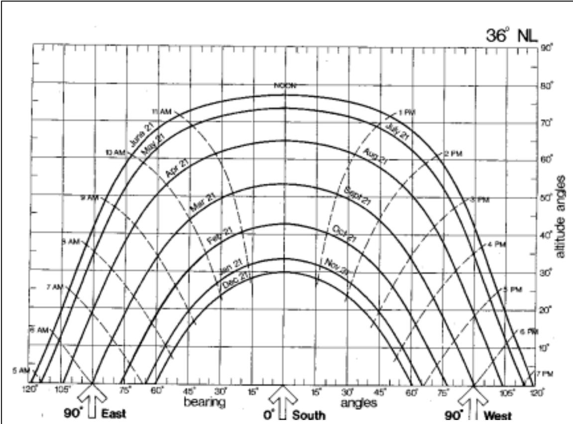
**Figure 3 Solar Path Chart for  $36^\circ$  North Latitude**
