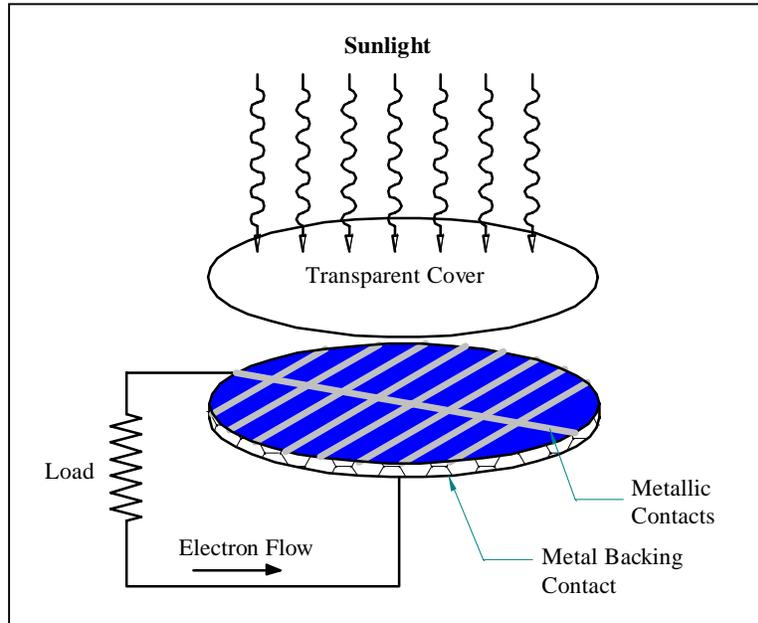
**Figure 15 Generic PV Cell and Circuit**
