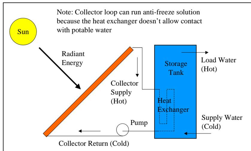
**Figure 8 Active Solar Heating System**
