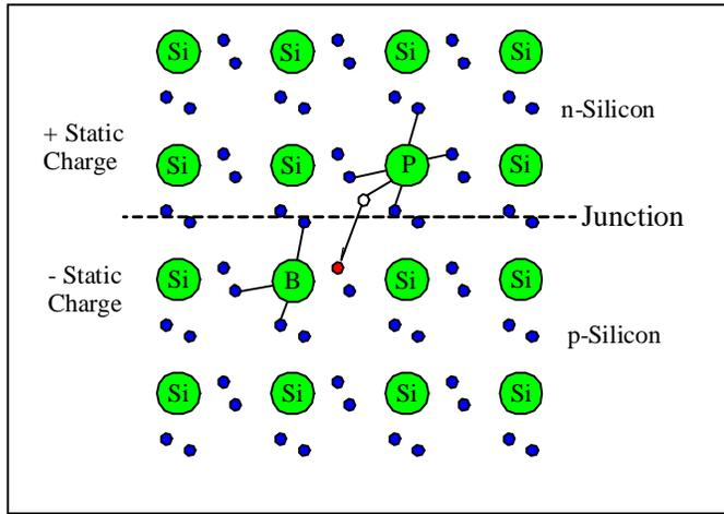
**Figure 17 PV Cell Junction**
