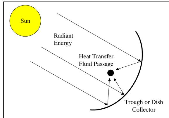
**Figure 12 Concentrating Collector**
