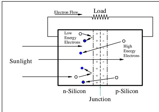
**Figure 18 PV Circuit Operation**
