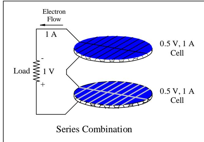
**Figure 19 PV Cell Voltage Addition**
