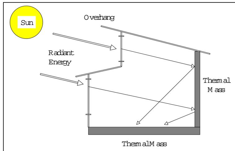
**Figure 10 Passive Solar Construction**
