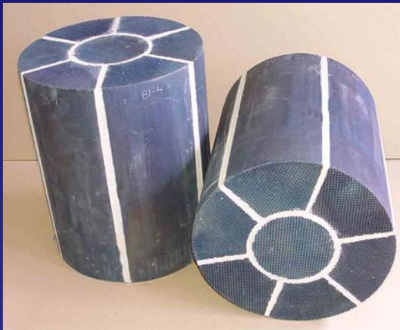
Diesel Particle Filter for a city bus
