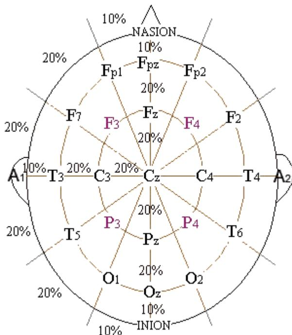
Figure 2: 10-20 electrode placement system for EEG measurement
