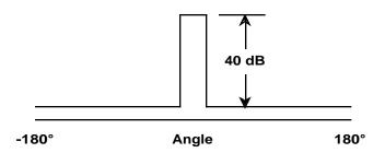
In this case there will be a contribution to the antenna noise temperature from the (attenuated) background noise temperature in the backlobe direction, and also a minor contribution from the sidelobes directed at the sky noise. As an example, consider the contribution of black body radiation from the surface of the earth at  $T_p = 290^{\circ}$ K occupying 180° of the sidelobe angles (1/2 the entire solid angle of the antenna radiation sphere).
