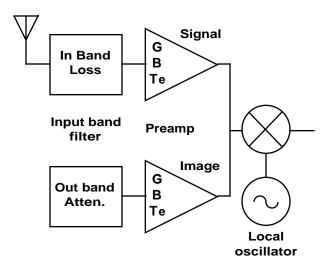
An equivalent circuit shows both the signal frequency and image frequency contribution to noise. The gain and noise temperature of the preamplifier will typically be different for the two frequencies, with the higher frequency generally exhibiting lower gain and higher noise temperature. In the more general case, there is possible noise contribution at higher order mixer harmonics spurious frequencies.
