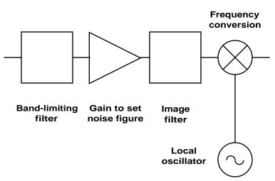
Note also that oscillator noise is impressed on signals, which creates a dynamic range issue to be treated elsewhere.
