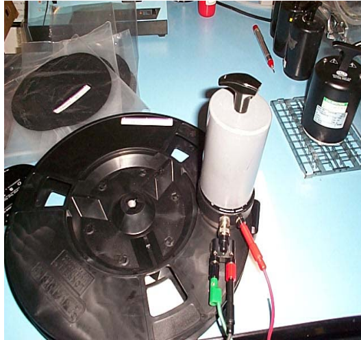
Figure 6. Measuring Resistance on the Outer Surface
