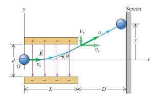
**T7.2** Electrostatic deflection of an electron beam in a cathode-ray tube.
