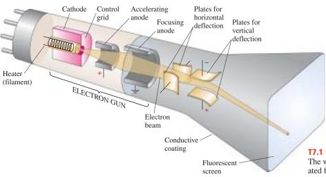
**T7.1** Basic elements of a cathode-ray tube. The width of the electron beam is exaggerated for clarity.
